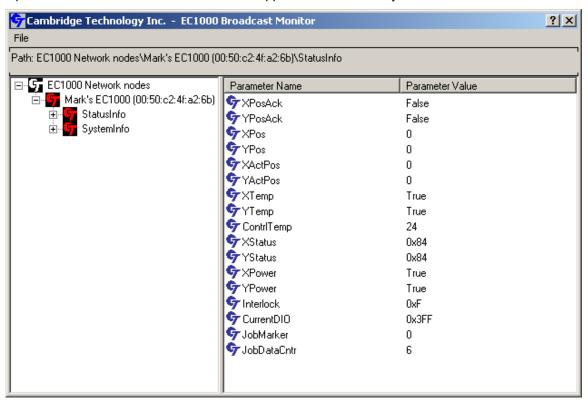
The Broadcast Monitor is used to identify all the EC1000's accessible from the system and it provides data about the EC1000s to the RTC Emulation DLLs. If you see a display similar to the image above, then your EC1000 is visible to the software and you can proceed. You can minimize the Applet by selecting the menu item File→Hide.
